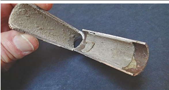
Figure 3: CaCO 3 scale in an extracted and bisected heat exchanger tube [4].
